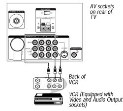
You can view the playback of VCR tapes (Video Disc players, camcorders, etc.) by using the AUDIO and VIDEO INPUT sockets on the rear of the TV.
